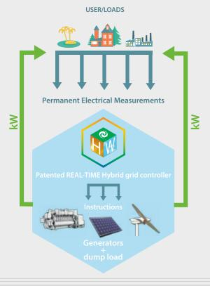
Hybrid Wizard<sup>™</sup> integrates a smart management system based on a permanent feedback loop, circulating throughout the system. By constantly monitoring the grid parameters, Hybrid Wizard<sup>™</sup> is able to send individual instructions to all generators, to automatically optimize the system, in real-time.
