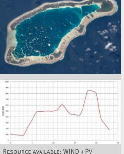
RESOURCE AVAILABLE: WIND + PV Payback time: 6.3 years Diesel saved: 245 000 Liters/year LCOE Hybrid: - 13% vs all HFO+diesel cost
